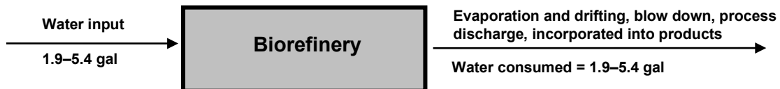
FIGURE 21 Water Input and Consumption for a Biorefinery Producing One Gallon of Cellulosic Ethanol, before Co-Product Allocation. (The values decrease to 1.9–4.6 gal when water use attributable to the excess electricity generation is considered.)
