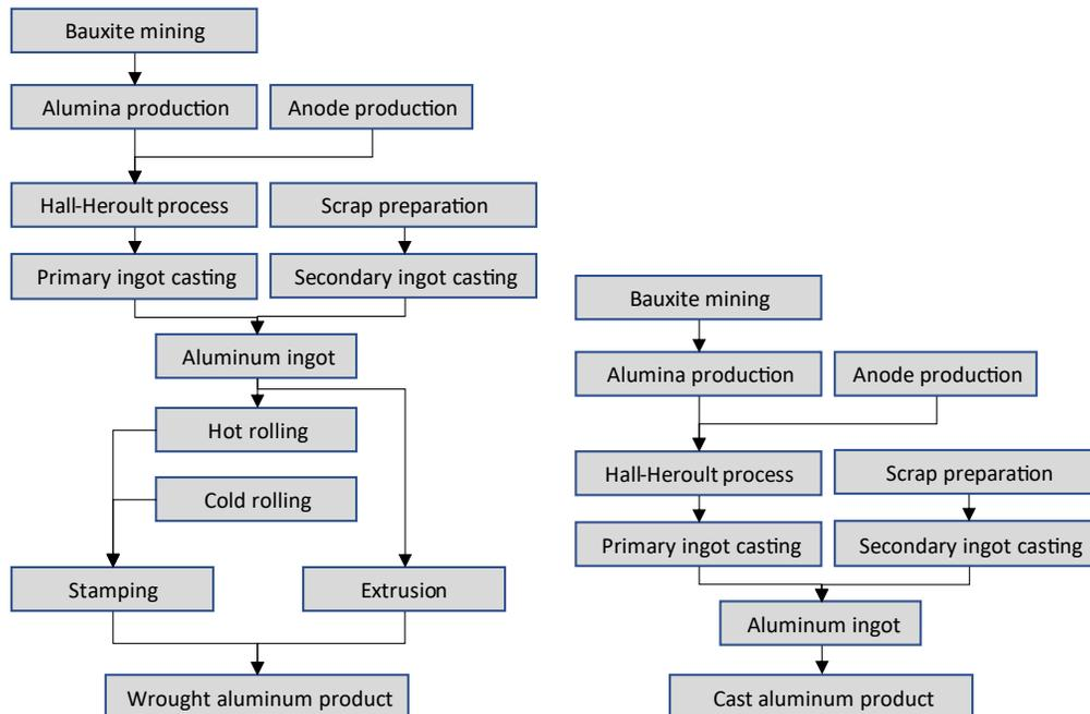
**Figure 16. Wrought and cast aluminum production steps**
