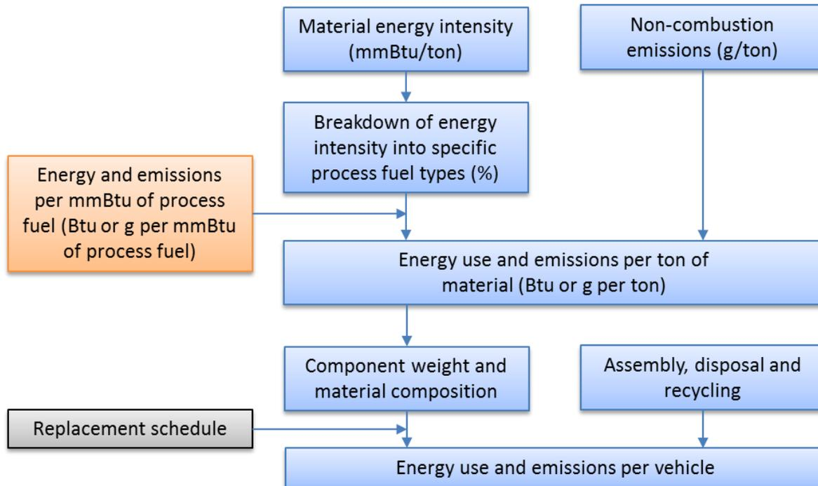
Figure 14. Process for GREET vehicle manufacturing cycle analysis
