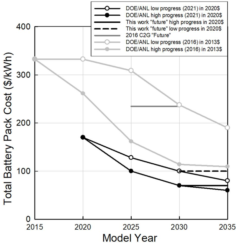
**Figure 12. Total battery pack manufacturing cost estimates assuming high (filled symbols) and low (open symbols) progress from DOE/Argonne in 2016 (grey lines, Moawad et al., 2016) and in 2021 (black lines, Islam et al., 2021). FUTURE TECHNOLOGY case values used in our previous C2G study (Elgowainy et al, 2016) and in the current work are shown by horizontal lines. The CURRENT TECHNOLOGY costs used in our previous and current work are shown where the lines converge.**
